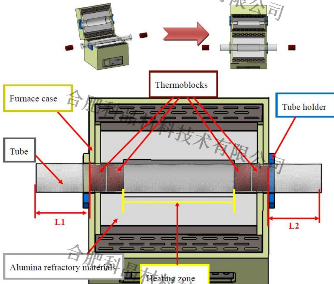
Our high temperature OTFseries (for 1500°C grade and up)furnaces require two thermoblocks on each side.
