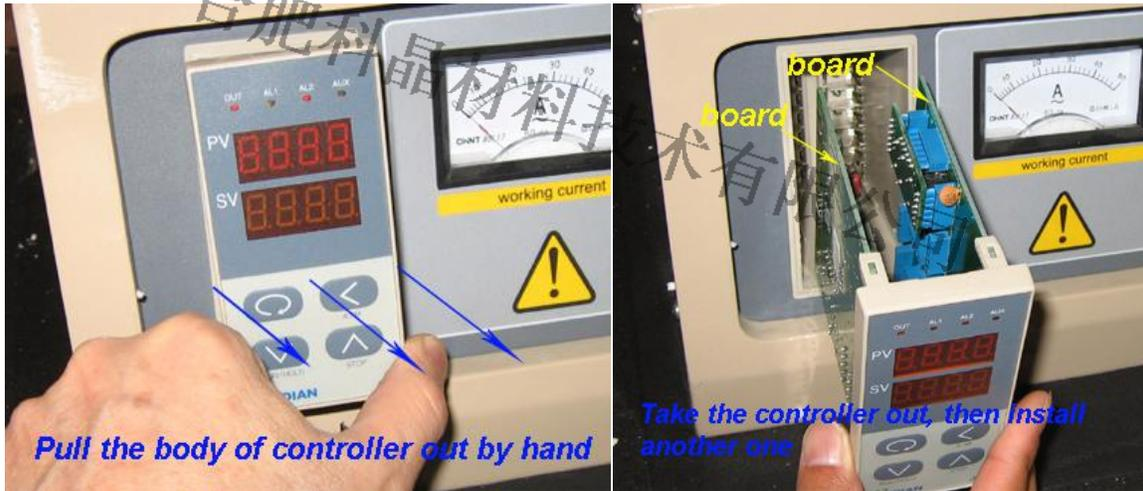
**Fig.3** uninstallation of temperature controller, step 2 and step 3
